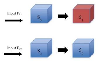
A computation is the result of a **change of state** of a given physical system, under the action of an external force.
